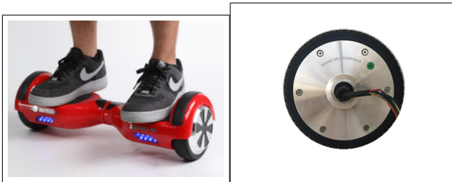
Figure 1.6: Self Balancing Scooter driven by BLDC motor
