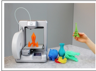
Figure 5.1: A Fused Decomposition Modeling rapid Prototyping Machine with the created objects
